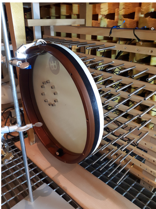
FIG. 2. (Color online) Modified frame drum positioned in front of the microphone array.
